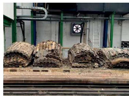
Denatured material after the 24 hour process. Once the material has cooled it is removed from the kiln and crushed to produce the recyclable aggregate.
