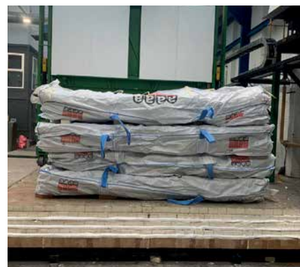
Asbestos cement sheets are delivered from construction sites to the treatment plant in specially designed easy to load bags.
